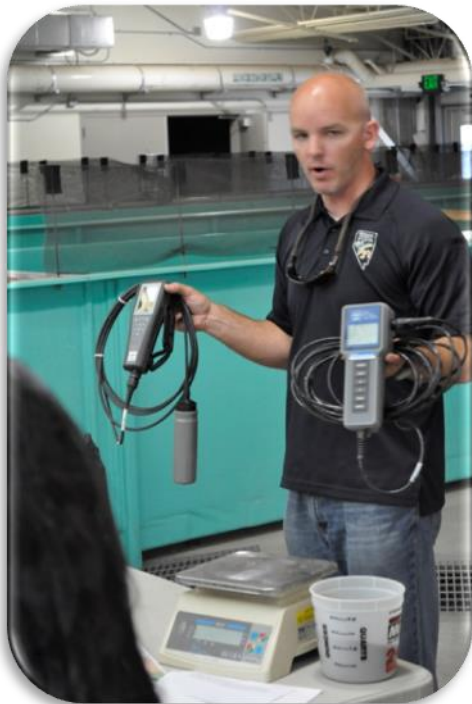
Figure 1.—Todd Wright of the NDOW demonstrates how water quality is monitored in hatchery raceways.
