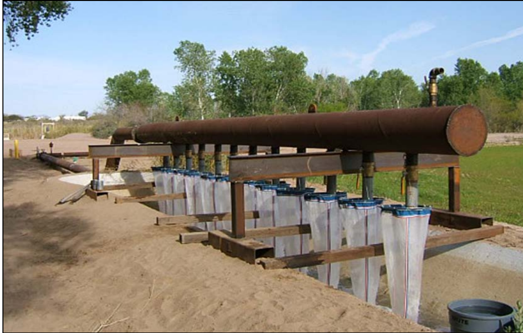
Figure 3. The large steel manifold with 12 evenly spaced sampling ports and attached plankton nets. Photograph taken during the 2009 evaluation (McDonald and Karchesky 2010).
