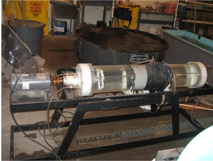
**Figure 3.—Swim chamber used to measure failure velocities.**
