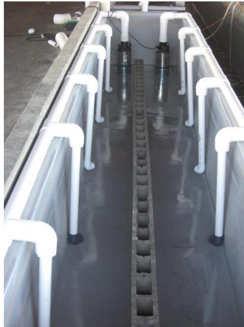
**Figure 1.—TR 1 raceway design utilizing PVC returns.**
