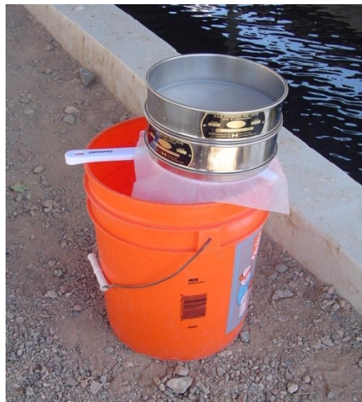
Figure 2. Removal of larger algae from collection sample using a 250- \mu m and a 212- \mu m sieve set above a 35- \mu m mesh net.
