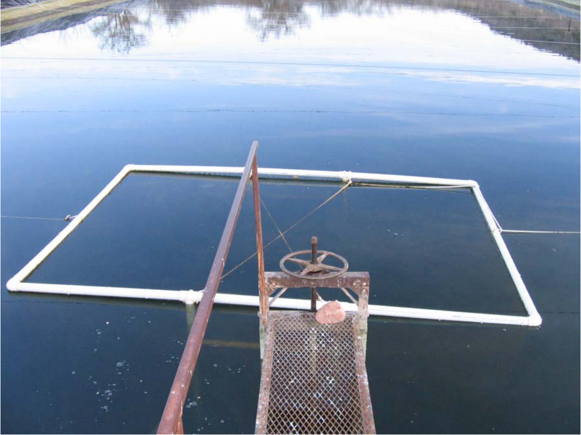
Fig. 2. Subsurface pond feeder deployed at Bubbling Ponds State Fish Hatchery, Cornville, Arizona, as viewed from the feeding catwalk. Exclusion consists of a PVC frame lined with 2.54-cm hexagonal mesh, galvanized poultry netting. Food is distributed to the surface (within the PVC) and is allowed to sink to a depth of 1.83 m before consumption is possible.
